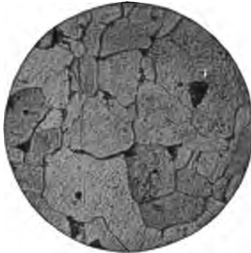
Fig. 28. Crystalline Structure of Overheated Steel
